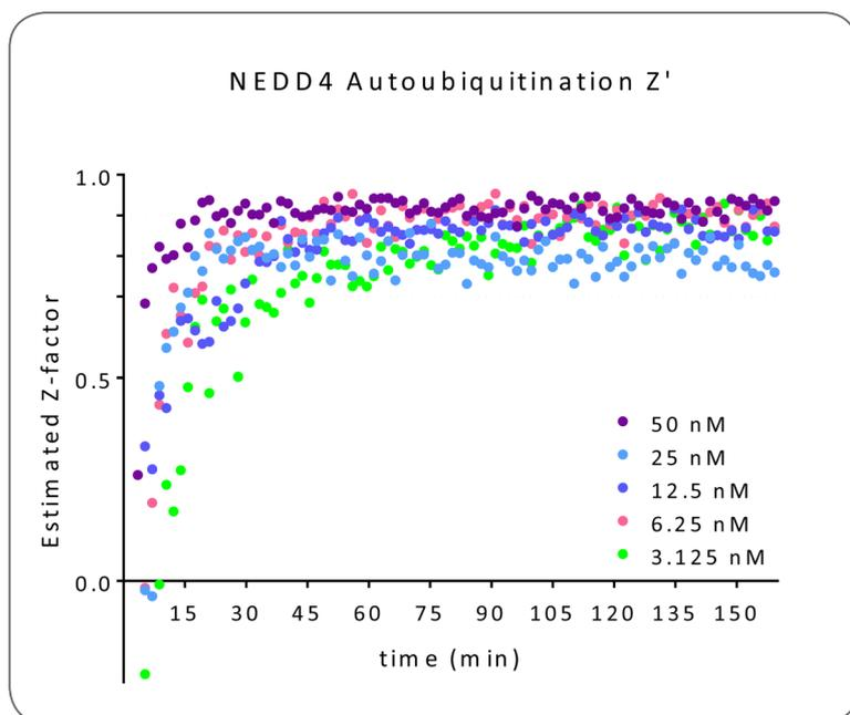
**Estimated Z-primes of Continuous Real-Time TR-FRET MDM2 titration (auto-ubiquitination):** Serial dilutions of NEDD4 from 50 nM to 3.125 nM mixed with UBA1, UBE2L3, and trf-Ubiquitin mix. Reactions were initiated with addition of Mg-ATP.
