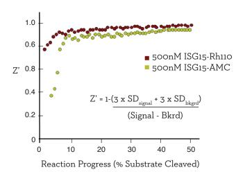
Robustness of Rhodamine110 vs 7-amino-4-methylcoumarin (AMC) substrates in an HTS format.
